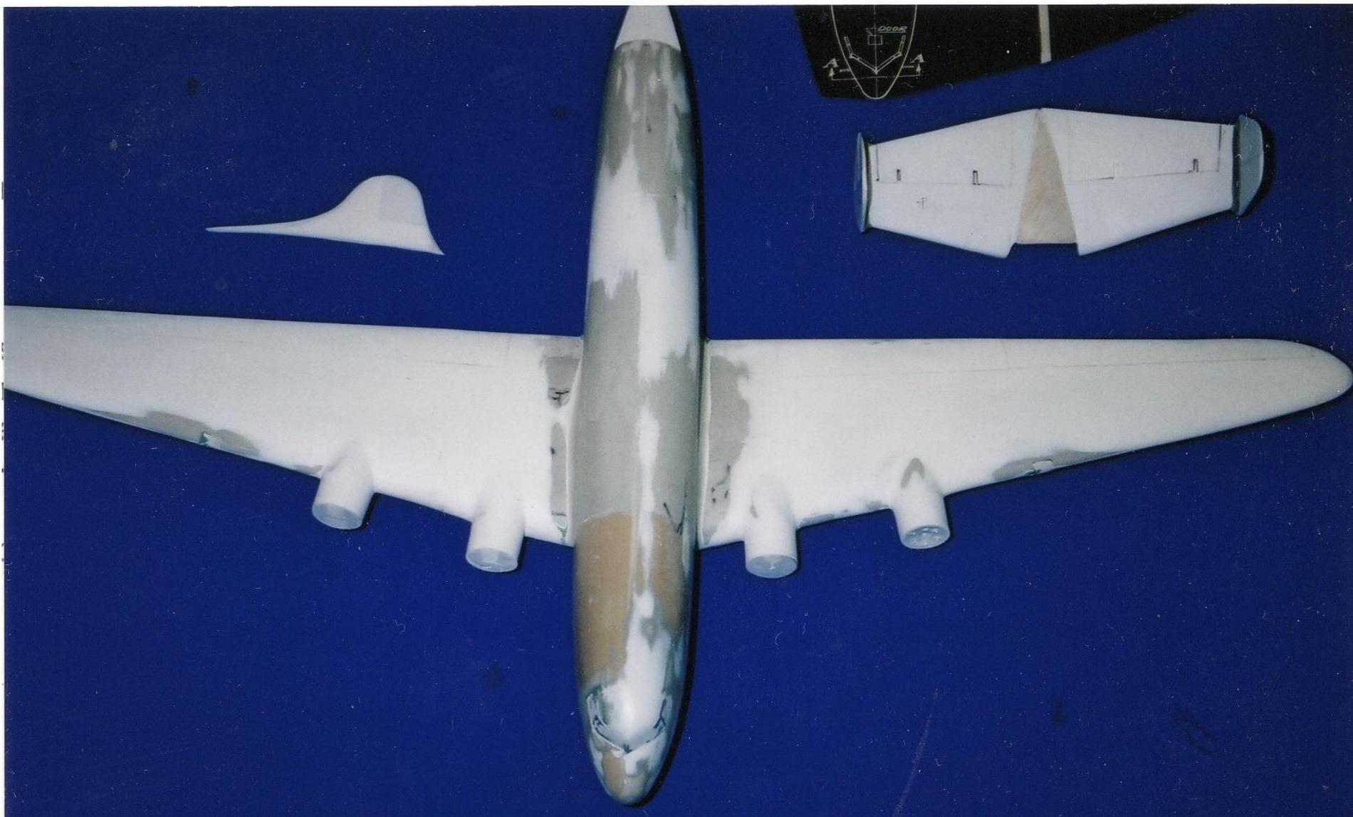
5- The fuselage sides are boxed together just like the wings were. After detailing the cockpit interior, the clear windshield with top is faired in place. The nacelles are made from rolled .030 styrene and are attached to the protruding stubs, which are canted outward on the DC-4E. Filled with Magic Sculpt, the nacelles are then blended into the wing.
