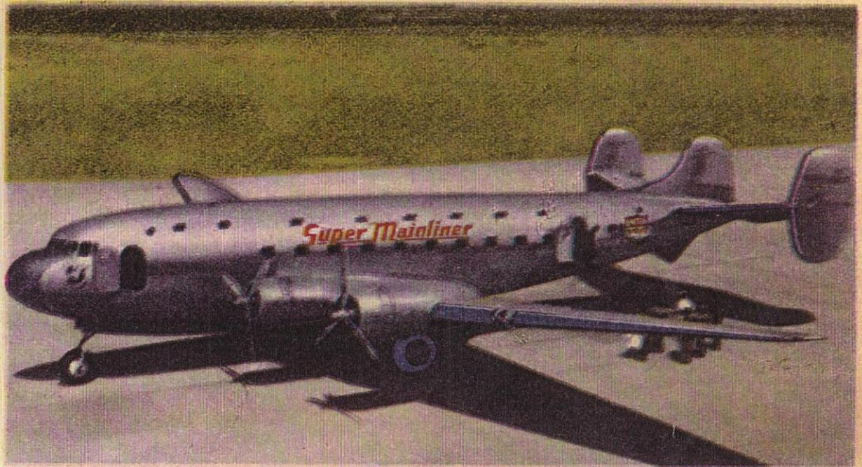
**PERFORMANCE** — Powered with four Pratt & Whitney twin-row "Hornet" engines developing 1100 h.p. each, the DC-4 has a maximum speed of 257 m.p.h., a cruising speed of 235 m.p.h. and a cruising range of 2600 miles. Rate of climb 1200 ft./min. Service ceiling 22,900 ft. Manufactured by Douglas Aircraft Corporation, Santa Monica, California.
