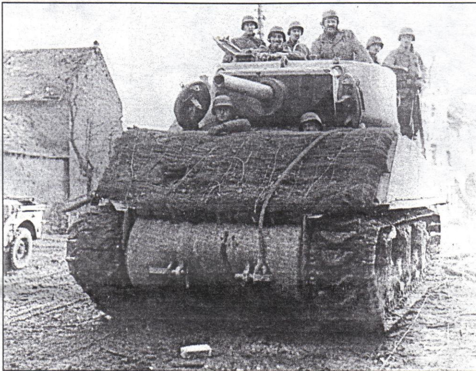
A Sherman Jumbo of the 743rd Tank Battalion near Altdorf, Germany on Nov. 27, 1944. The crew has sandbagged the glacis and then covered the sandbags with camouflage netting.
