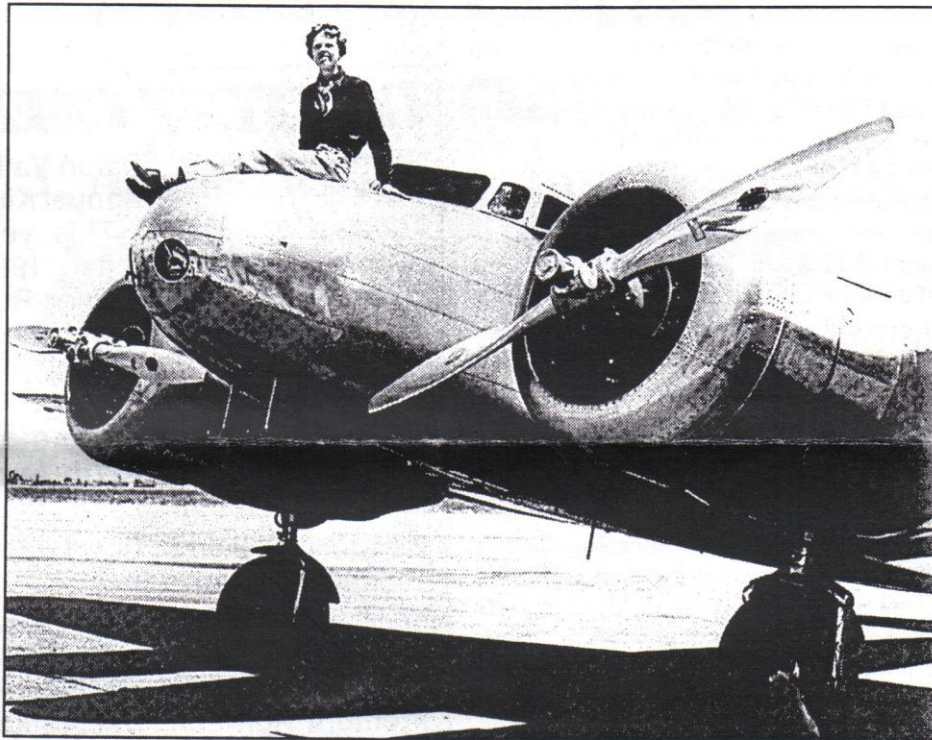
Amelia Earhart poses for a publicity photo prior to her 1937 round-the-world attempt. Modifications made to the plane boosted fuel capacity from 250 to 1150 gallons and stretched its range to 4000 miles.
