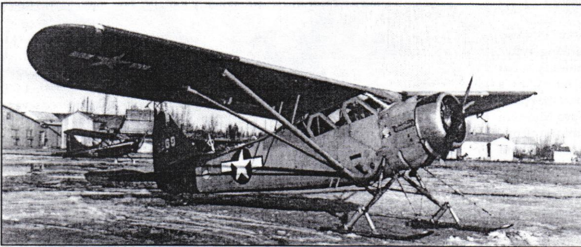
The versatile L-1 could function well on wheels, skis or floats, although only wheels are provided in the kit. Here is an L-1 based in Iceland in the search and rescue role.
