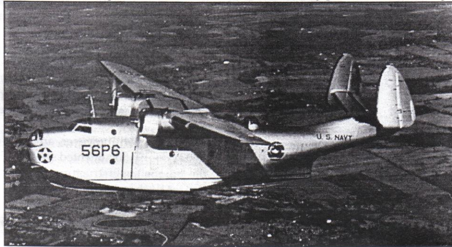
The first production PBM-1 in flight, 1940. This portly plane could lug a payload of four tons.
