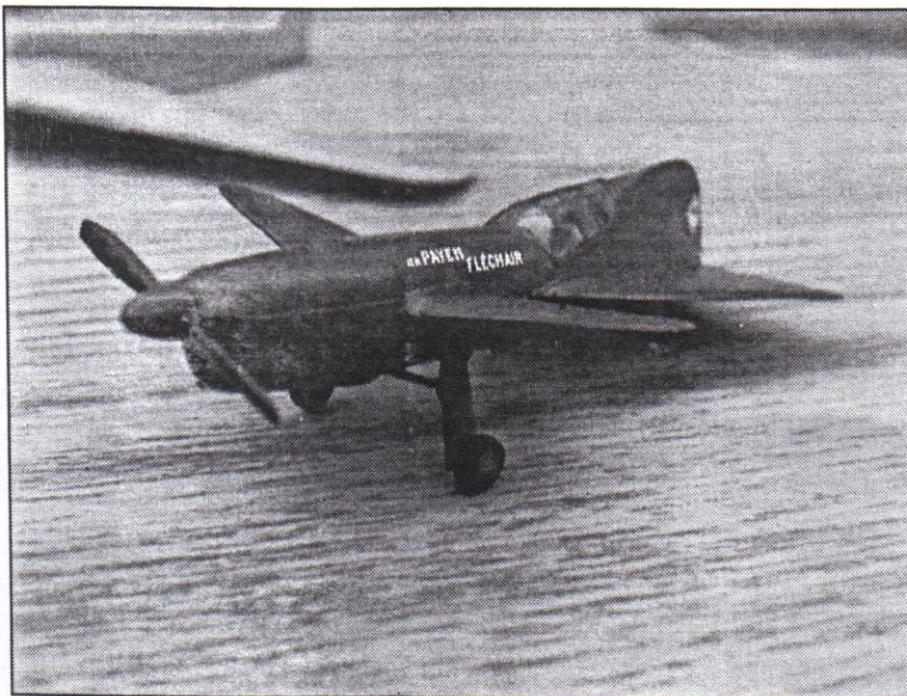
Ground-level shot highlights the fixed landing gear of the shark-like Pa.22.
