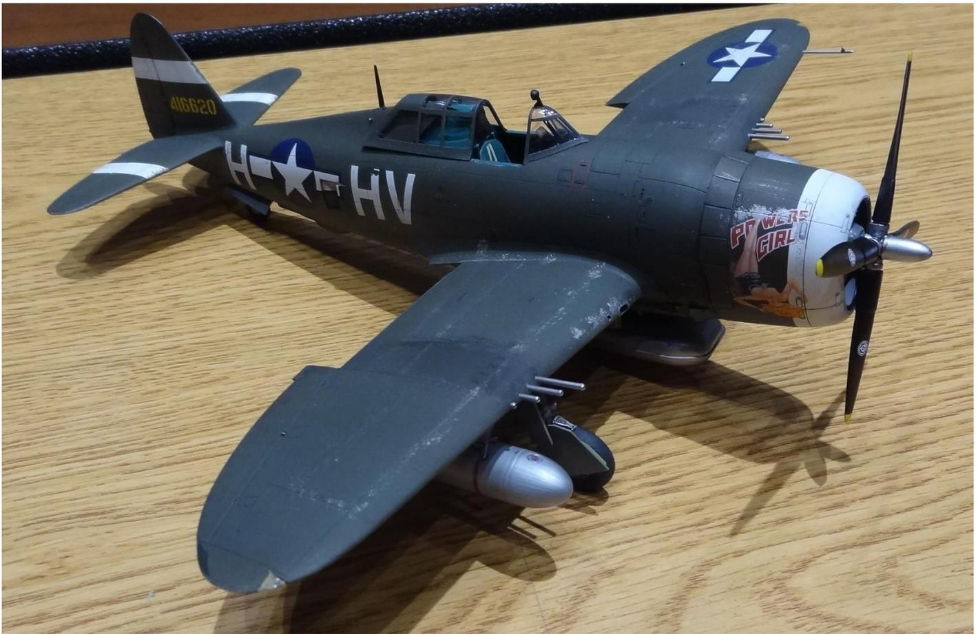
**Riley Kitchen's** Tamiya P-47D was finished as an early -D model with the "toothpick" propeller blades and looking lovely in a weathered scheme; Riley used MRP paints and weathered it with oils.
