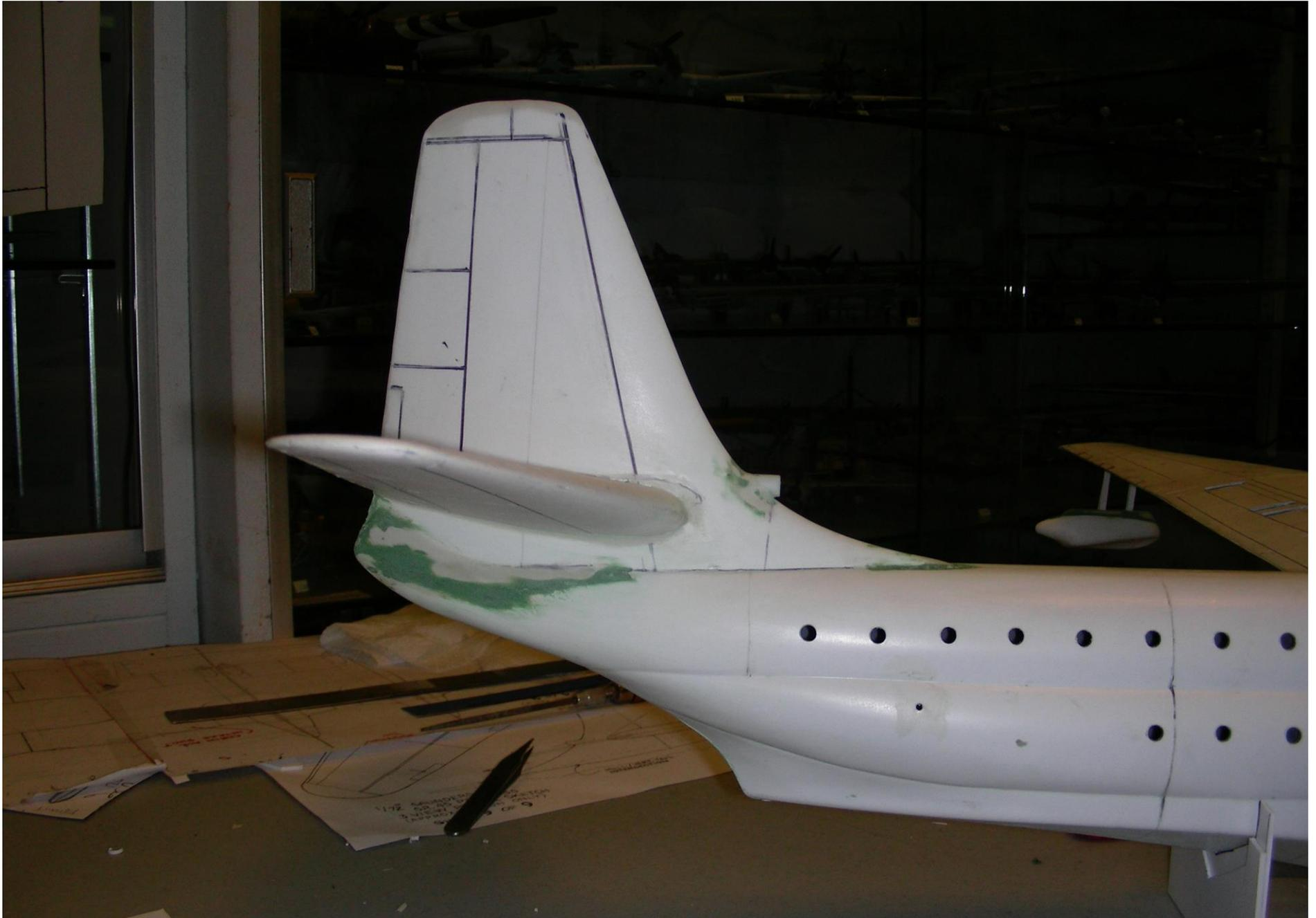
ANOTHER VIEW OF TAIL ASSEMBLY FIXED IN PLACE, FILLED AND SANDED AS NEEDED.
