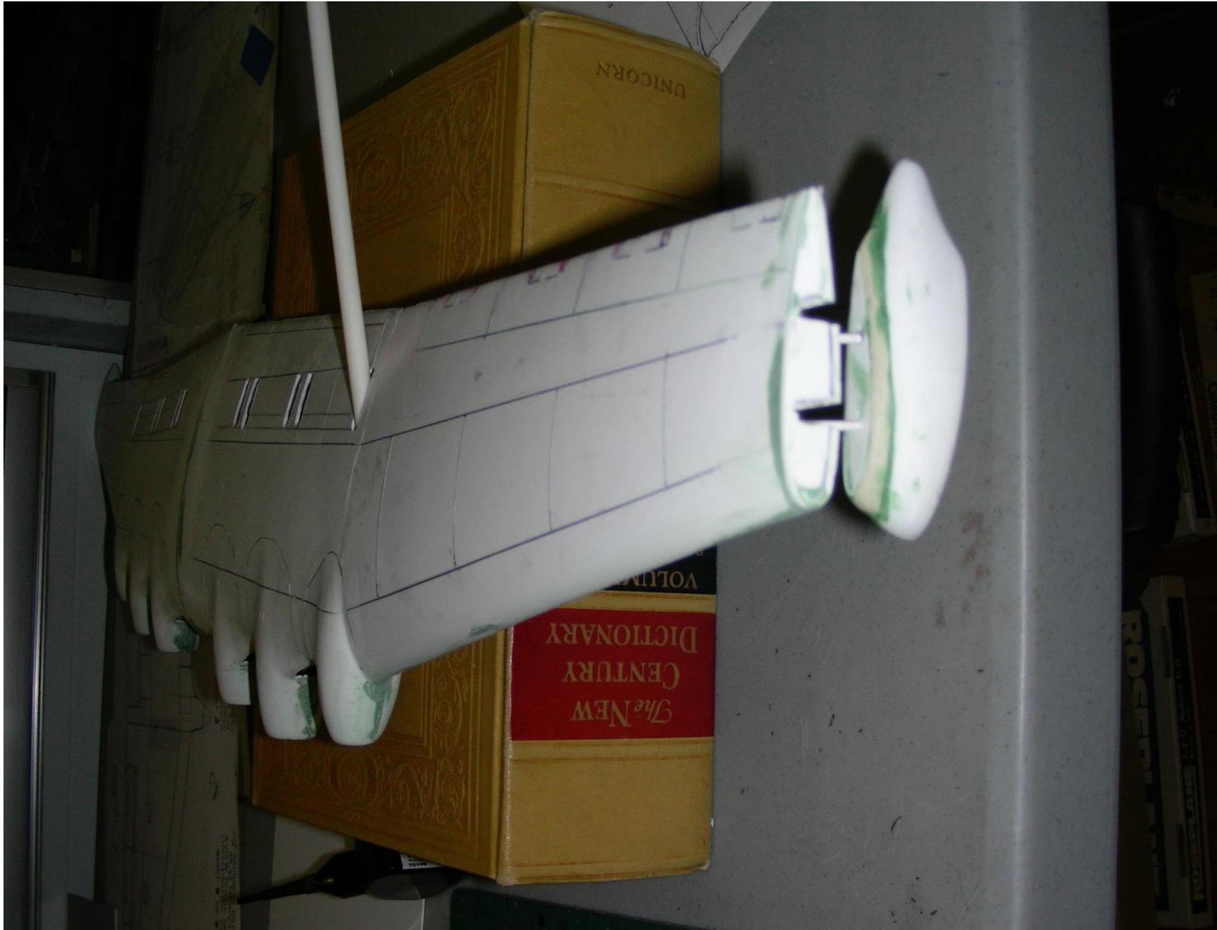
Here seen looking up at the bottom wing with the float in the retracted position. NOTE that the fairings have been bonded to their support wire snugly enough to hold firm in the retracted position and readily disengage when deployed.
