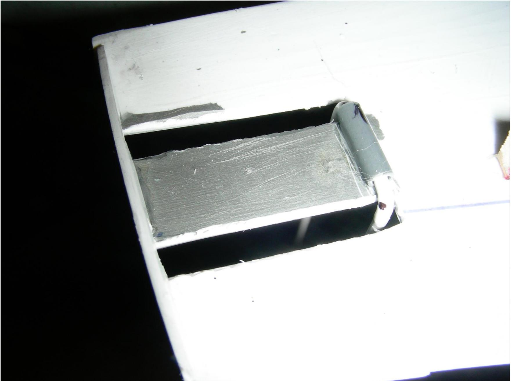
HERE we see the float attached to the wire and adjusted for fit before gluing. (make certain the float operates with precision before gluing the wire to the float). Once deployed the float will be held in place by gravity.
