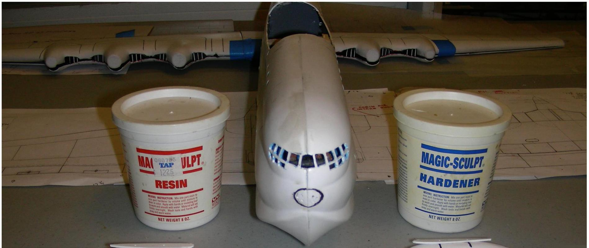
FRONT: Hull nose marked for radome. The 2 part resin is going to be used for creating the nose radome and front wing - to - hull fillets.
