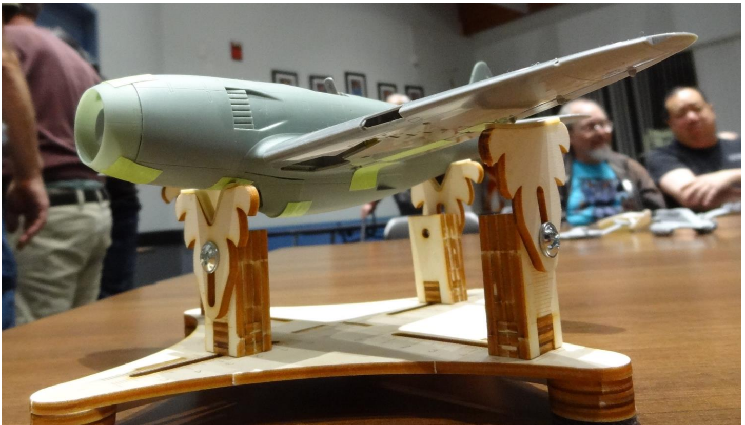
Mike Meek is using the Halberd conversion to change a Tamiya P-47 into the up-engined XP-72. The upgraded Thunderbolt differed in having an R-3350 engine and a different placement of the landing gear, in addition to other smaller changes.
