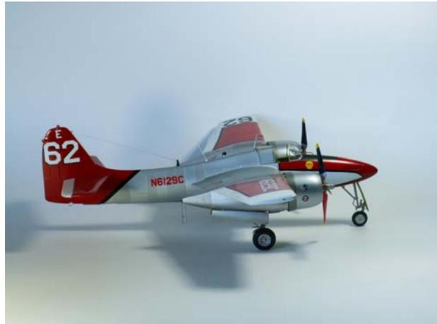
To get the model to set on its’ nose gear I placed lead “bb’s” right behind each engine nacelle, and on the inside bottom of the fuselage just behind the nose gear. The model is very heavy to say the least. So far the nose gear has not bent after almost two years.
